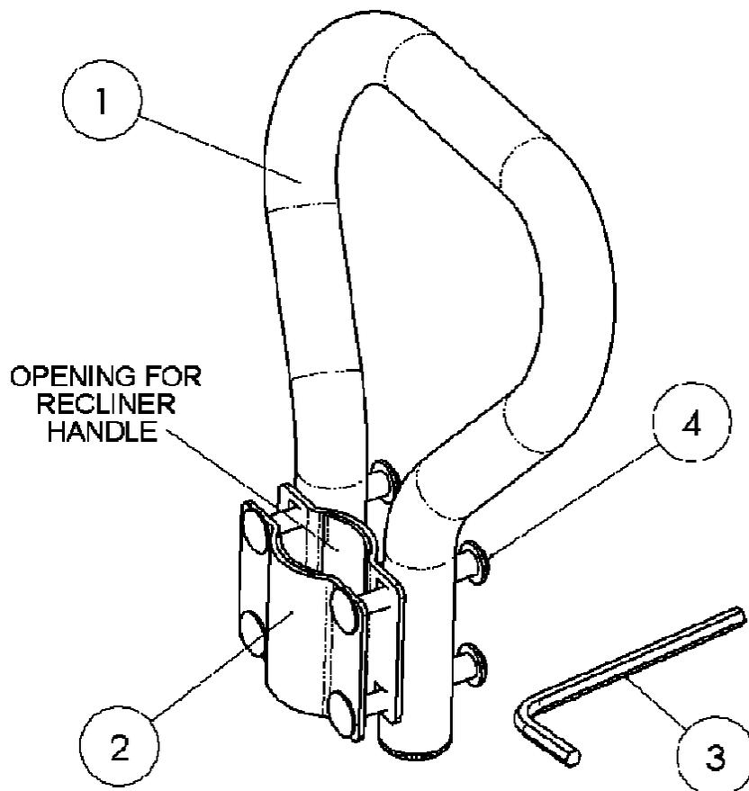
1. Loosen the four Bolts (Item-4) using Allen Wrench (Item-3) to allow Handle (Item-1) and Bracket (Item-2) to move apart from each other. This will create an opening between the Handle (Item 1) and the Bracket (Item-2). **Note: Just loosen the bolts, do not take bolts completely out.**
